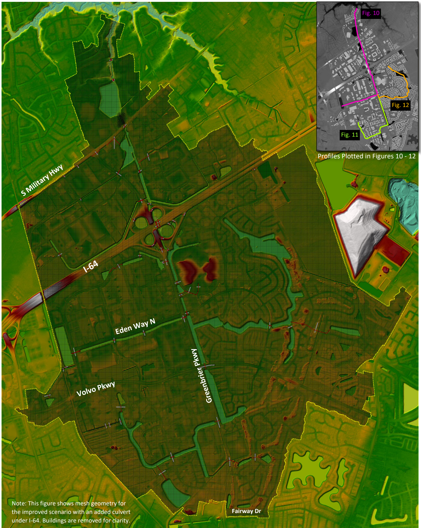
Figure 5. Rain-on-Grid Model Construction, 2D Mesh Geometry
