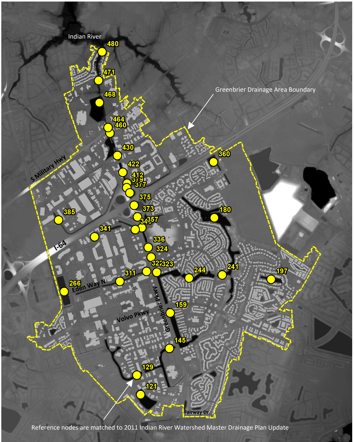
Figure 1. Greenbrier Drainage Area with Reference Nodes
