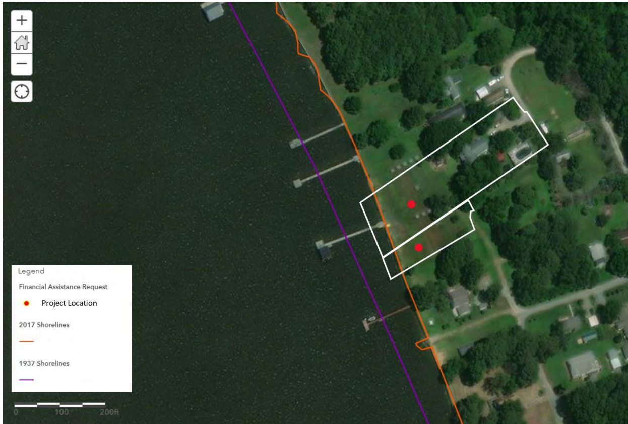
FIGURE 7: PROJECT LOCATION AND MAP OF THE SHORELINE CHANGE BETWEEN 1937 AND 2017. PLEASE NOTE THAT THE PROJECT AREA PARCEL IS OUTLINED IN WHITE.
